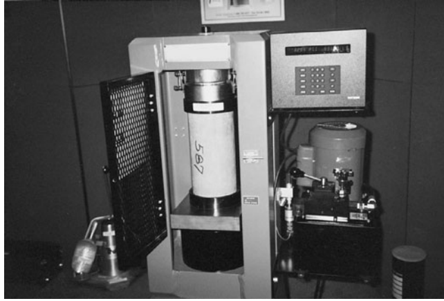
FIGURE 2.3 Testing a 6 × 12 in cylinder in compression. (Courtesy of the Portland Cement Association.)
